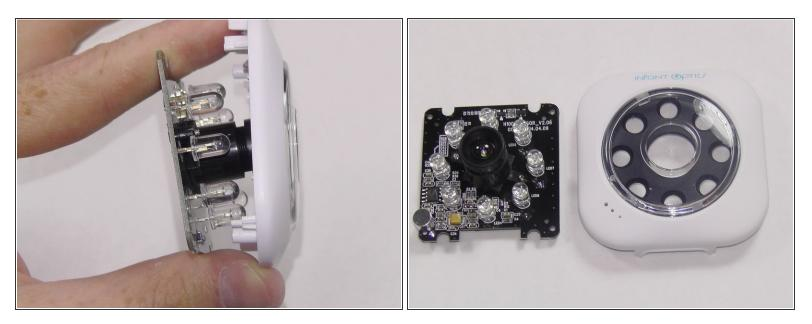
• Remove the front face plate of the camera unit by carefully pulling it off.
