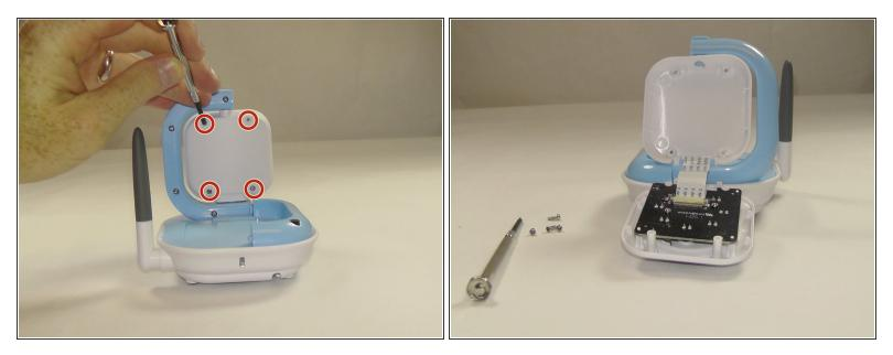
Using a Phillips #2 screwdriver, remove the four, 6.0 mm Phillips screws from the back of the camera unit.
