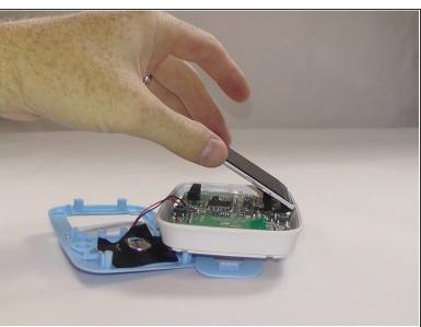
Carefully open the hand held monitor and flip the screen (highlighted in red) out of the way.
