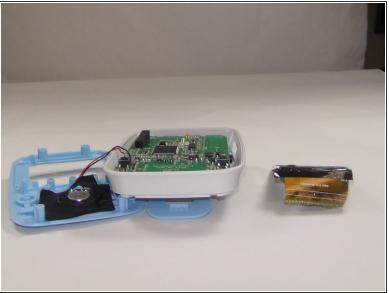
Remove the hand held monitor screen from the mother board by carefully pulling from the point where it is attached with an adhesive to the mother board.
