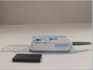
Remove the battery by pushing in on the right side and then pulling the battery up and out of the body of the hand held monitor.
