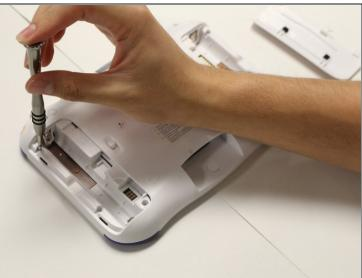
• Remove six 7 mm screws from the interior of the battery compartment using a Phillips #1 screwdriver.
