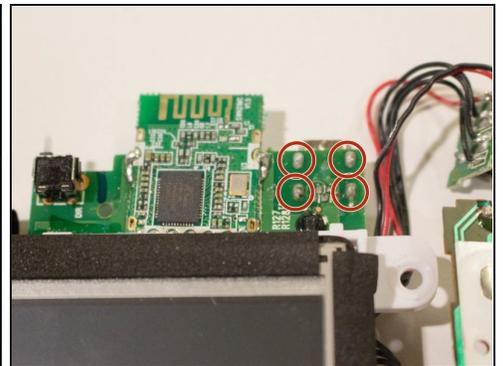
ⓘ The mini USB port is located near the top of the device and is secured by four metal prongs underneath the port.
