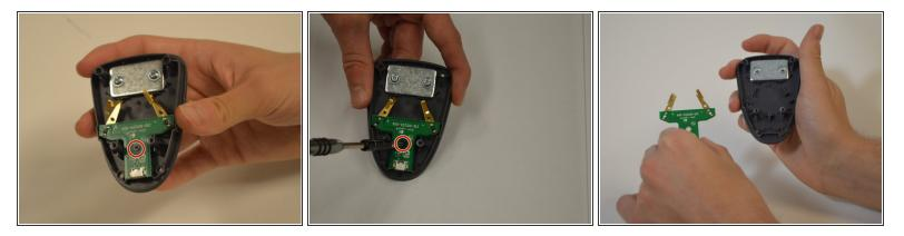
Use the Phillips #0 screwdriver to remove the last (4mm) screw. The motherboard can now be removed.
