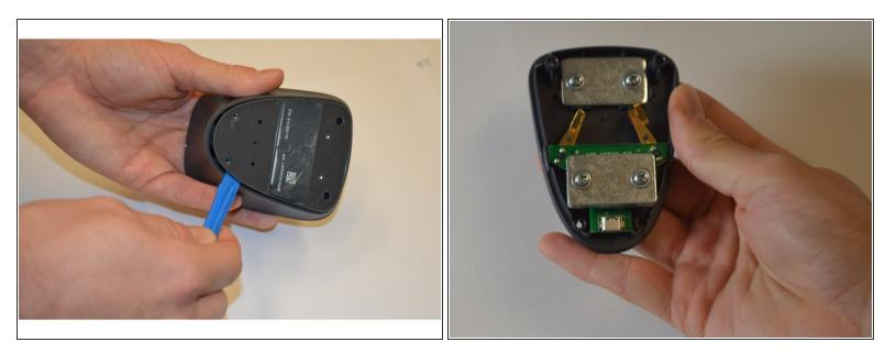
• Use the plastic opening tool to remove top shell from device.
