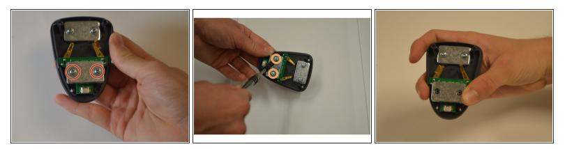
• Remove the two (4mm) screws using Phillips 1 screwdriver.
