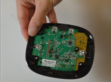
Use a plastic opening tool to remove the top shell of the device.
