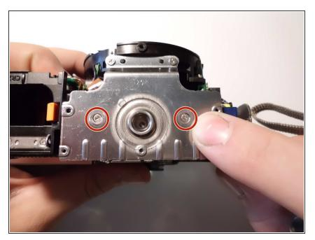
• Remove the two silver 1mm screws on either side of the tripod mount.
