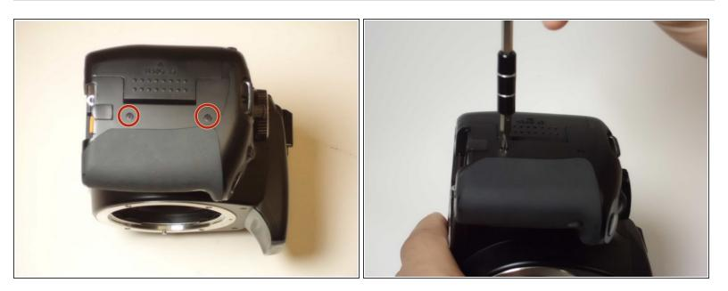
• Remove the two black 6 mm Phillips screws from the right side of the camera.
