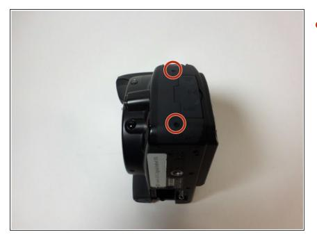
Remove the two black 4 mm Phillips head screws on the side of the camera opposite to the hand grip.
