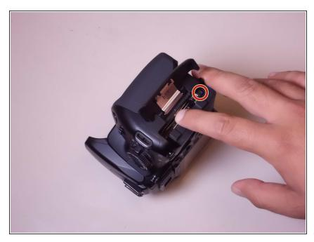
• With the door open, push down the small black plunger next to the CF slot. The CF card will disengage from the slot and be ejected far enough that you can grasp it between thumb and forefinger and remove it from the slot.
