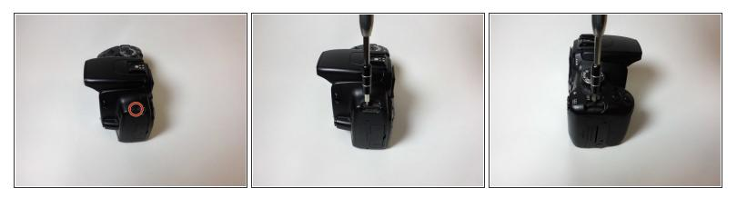
• Remove the two black 4 mm Phillips screws on each side of the camera under the strap hooks.
