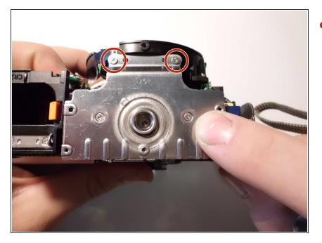
Remove the two silver 6 mm screws towards the front of the camera on the tripod plate.
