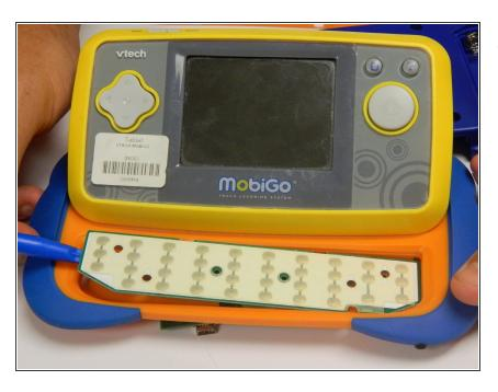
Gently remove the keyboard circuit board with a plastic opening tool.
