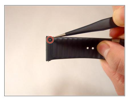
Remove the wristband by sliding the metal pins located on both sides of the wrist band, and pulling the wristband off.
