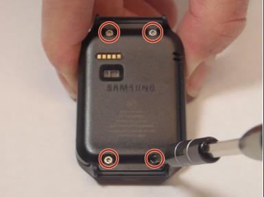
• Use a T5 Torx Screwdriver to remove the 4 (0.4 mm) screws located on the back of the watch.
