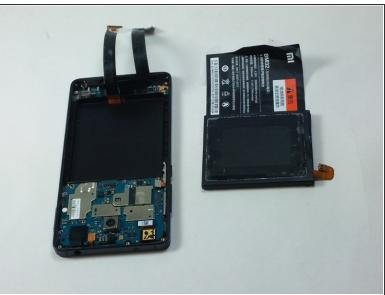
Use the plastic opening tool to gently pry the battery out of its casing for removal.
