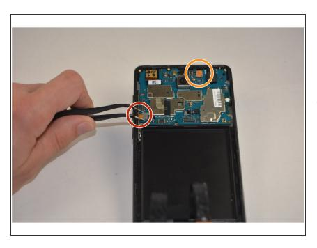
With the battery removed locate the left-hand cable connected to the motherboard. With the tweezers,
