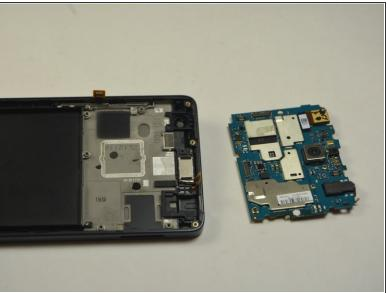
Wedge the plastic opening tool, between the motherboard and the inner region of the phone in the slot atop the motherboard.
