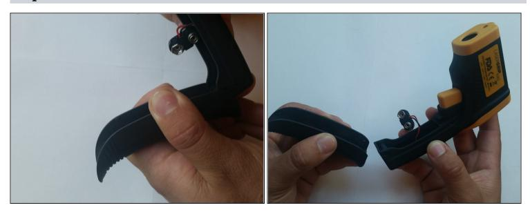
• Remove the battery cover from the device by pulling it straight out.
