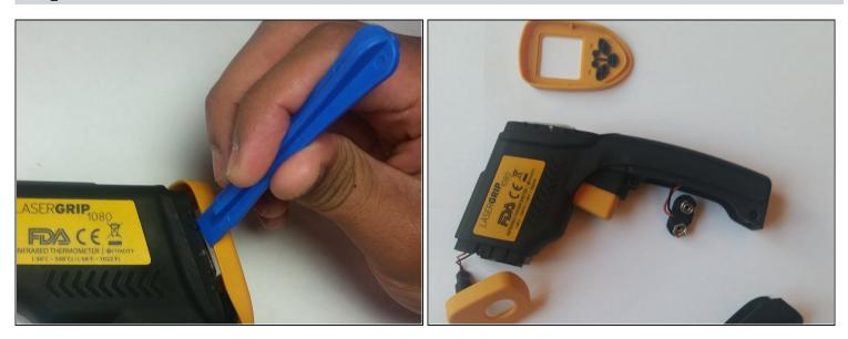
Using the plastic opening tool remove the front and rear yellow covers.
