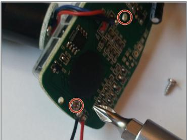
• Unscrew the two 3.4 mm screws on the motherboard.
