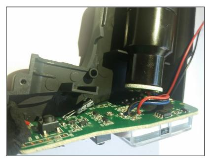
• Pull the motherboard out of its slot in the device.
