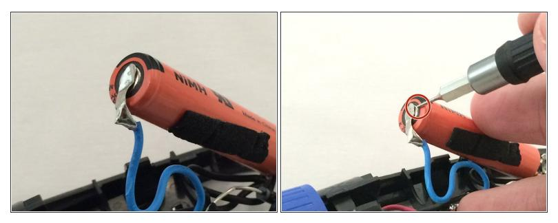
Locate the connection between the blue wire and the battery. Melt the solder and completely remove the battery.
