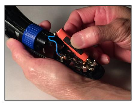
Grab the battery by its sides, pull it upwards out of the base of the trimmer.
