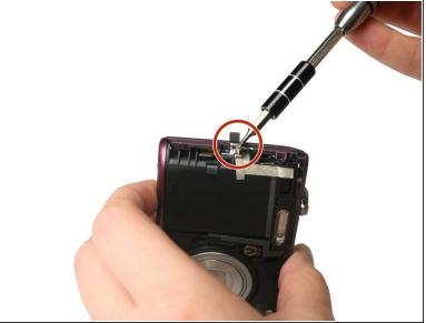
Using the Philips #000 head screwdriver, remove 2 additional 3.30 mm screws holding the lanyard mount in place.
