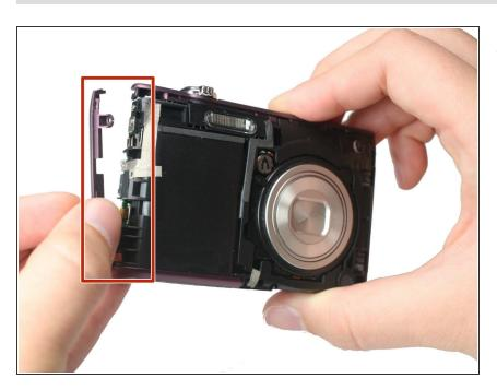
Remove the remaining side shell casing.
