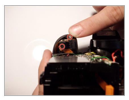
Use a J00 screwdriver to remove the two silver 4 mm screws from underneath the snapshot button.
