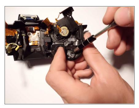
Use a 1.5 flat head bit to remove the c-clip from underneath the snapshot button by pushing against the open side of the pin.
