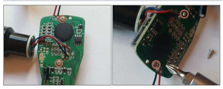
• Unscrew the two 3.4 mm screws on the motherboard.
