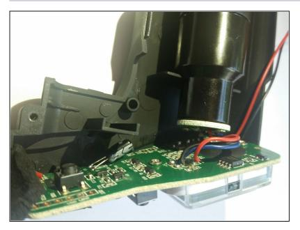
• Carefully pull the motherboard out of its slot in the body of the device.
