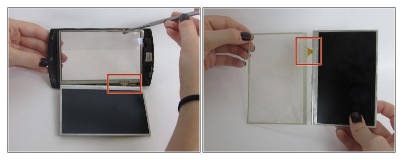
• Lift the cracked screen off of your Archos 5 using the regular plastic spudger.
