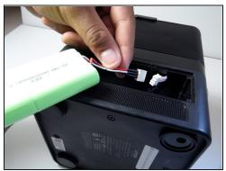
• To remove the battery, use one hand to pull on the battery wires, use <u>tweezers</u> to pull on the connecting head of the speaker.
