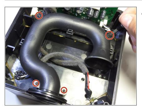
Remove the four 8 mm Phillips #1 screws.
