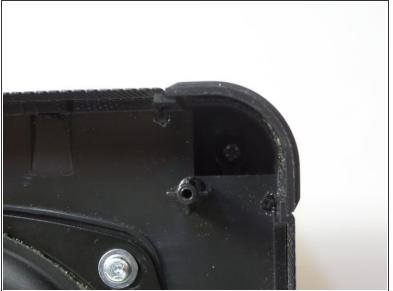
Remove the four 13 mm Phillips #1 screws.
