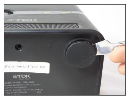
Remove the four rubber feet of the device using a metal spudger.
