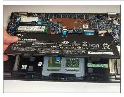
• Carefully remove the battery from the device.
