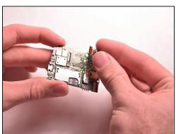
• Carefully wiggle the camera away from the device.
