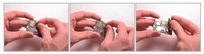
• Carefully wiggle the camera away from the device.
