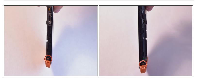
• Remove the two 5mm T4 screws on the sides of the small orange plate.
