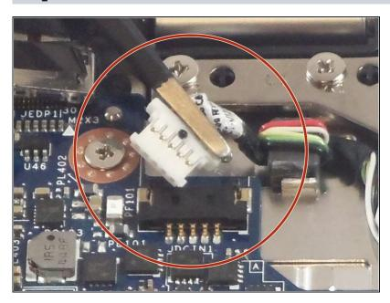
Use the tweezers to unplug the USB port from the motherboard by gently lifting the white connector up from the black motherboard connector.
