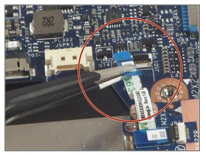
Use a pair of tweezers to disconnect the motherboardside of the SD board ribbon cable. Gently lift up the black tab, and then ribbon cable should come free from the ZIF connector.
