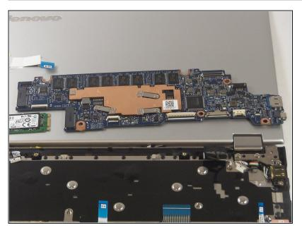
• Gently lift the motherboard up and out of the device.
