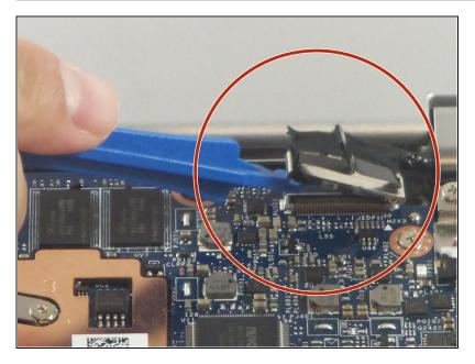
Use a plastic opening tool to gently pry up the screen cable from the motherboard.
