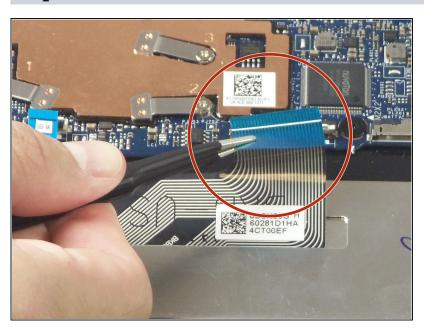
Use a pair of tweezers to disconnect the keyboard ribbon cable from the motherboard ZIF connector. Gently lift up the white tab, and the cable should come free.
