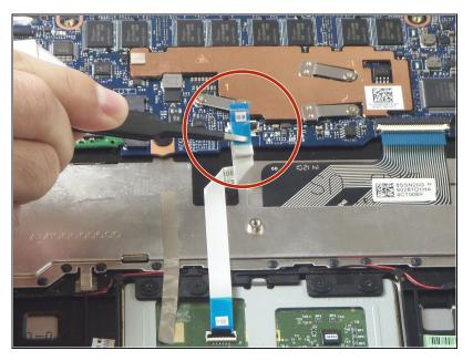
Use a pair of tweezers to disconnect the motherboardsize of the trackpad ribbon cable. Gently lift up the black tab, and the cable should come free from the ZIF connector.
