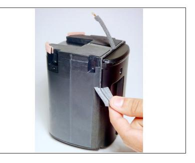
Using a plastic opening tool, remove the grey tape from both sides of the device.
