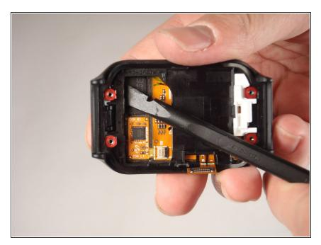
Once part of the display begins detaching from the front cover, place the spduger in between the display and the front cover.
