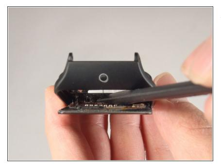
After the adhesive has been removed, apply pressure with the spudger to the back of the AMOLED display; the display should pop right out.
