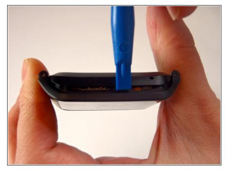
Slide the opening tool in between the two halves of the case and slide along the edge of the watch while gently prying the back cover away from the face of the watch.
