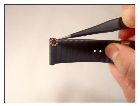
Remove the wristband by sliding the metal pins located on both sides of the wrist band, and pulling the wristband off.
