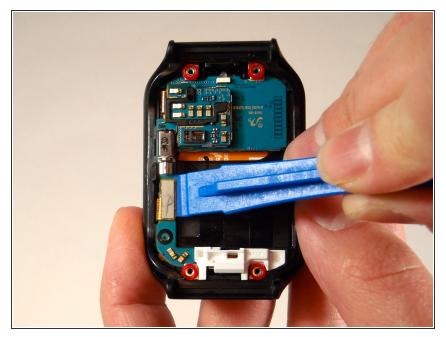
• Using the plastic opening tool, pull up on the flex connector. It will come off the motherboard, but will stay attached to the cover like a hinge.
