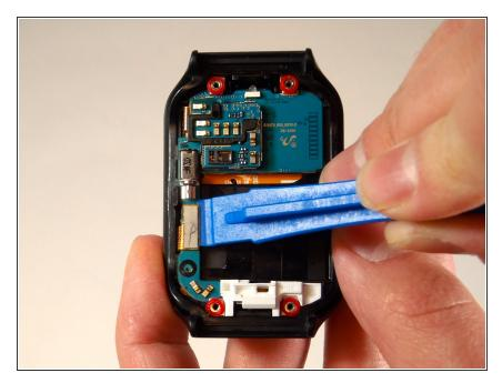
Using the plastic opening tool, pull up on the flex connector. It will come off the motherboard, but will stay attached to the cover like a hinge.
