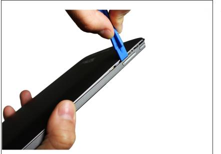
Use the plastic opening tool to work your way around the tablet, releasing the back case from the tabs.
