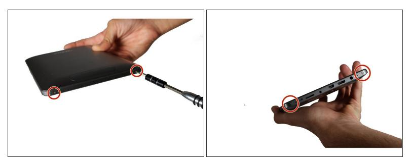
Remove the (4) 3.5mm screws using a phillips #000 screwdriver.
