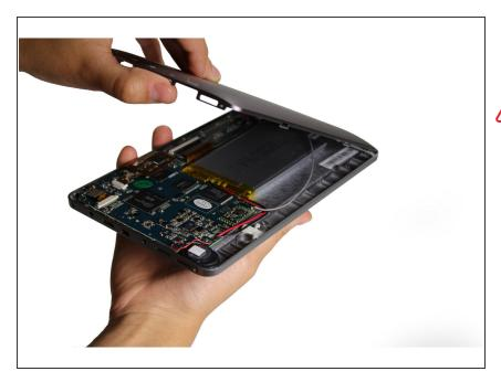
• Release the back case from the rest of the tablet with your hand.
