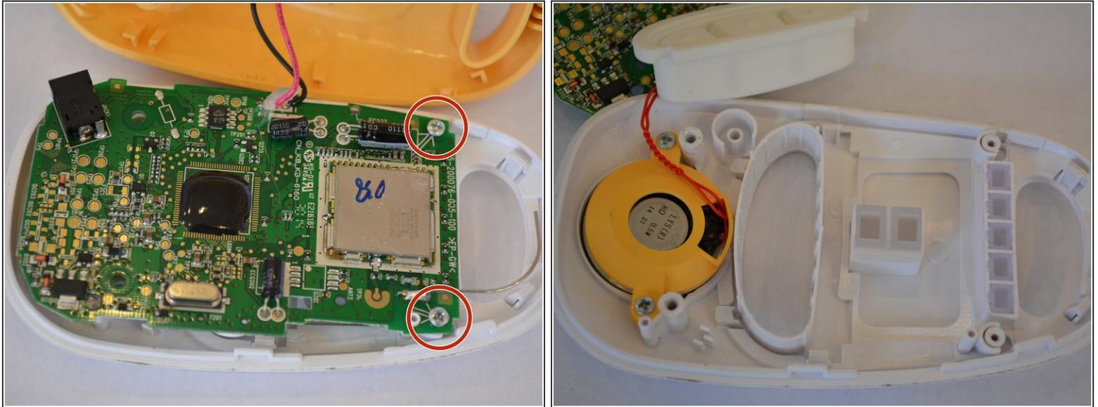
**⚠** When separating the motherboard from the front cover, be careful not to disconnect the two red wires which connect the speaker to the motherboard.
