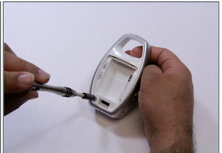
ⓘ There are two screws on the rare case of the device. For the one shown in blue marker requires either an extended screwdriver or putting on a little pressure on a regular screwdriver.
