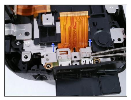
Lift up on the mounting bracket to remove the HDMI/USB Port from the camera.
