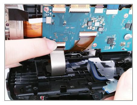
Disconnect the ribbon wire attaching the screen to the camera.
