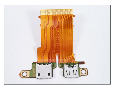
Once the HDMI/USB Port is removed the replacement can be installed.
