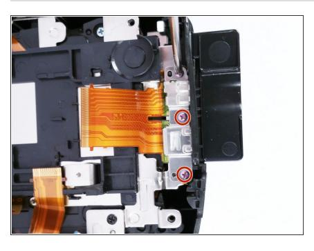
Remove the 3 (4 cm) Phillips head screws securing a mounting bracket over the HDMI/USB Port.
