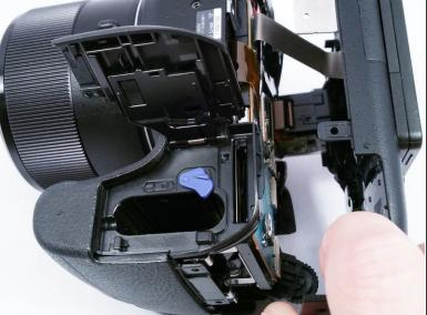
Using a plastic opening tool, separate the plastic camera housing.
