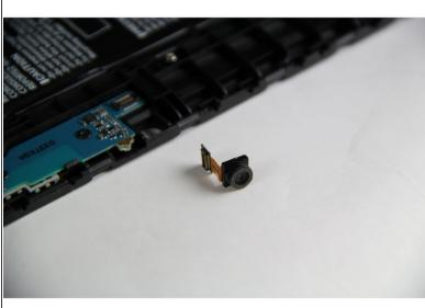
Pull the camera upwards to remove it from the device.
