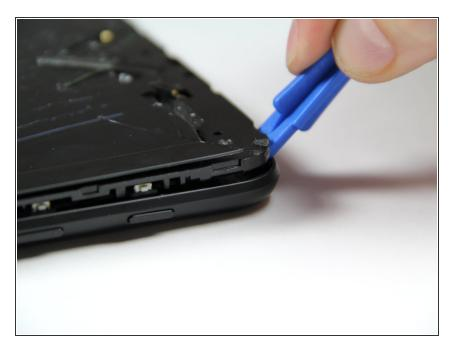
Once the edge of your device's panel is separate from the screen, continue moving around the outside of the device while continuing to pry the two pieces apart from each other.
