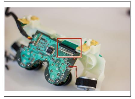
• Check the connection of the flexible trigger board to the main circuit board of your controller.
