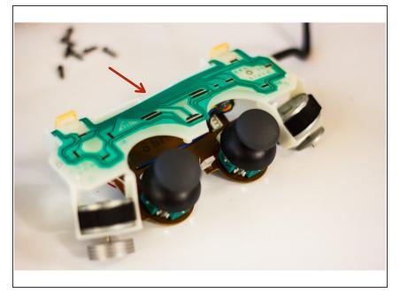
• Examine the flexible trigger board itself for any dirt or debris that could get in the rubber button pad's way.
