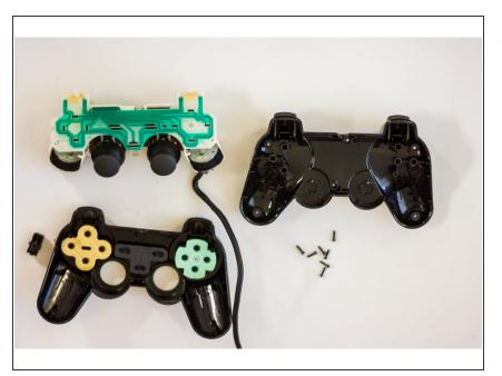
Carefully remove the circuit board from the front cover of the controller.
