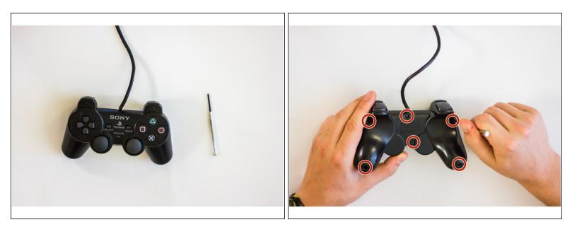
Flip Over Controller and remove all 6 screws from the bottom of the controller.
