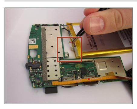
Once the wires have all been released remove the battery from the device and replace with a new battery. To reattach the new battery wires please refer to this guide on How To Solder
