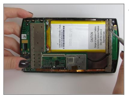
Separate the grey tape by using a plastic spudger. The tape is holding the battery in place.
