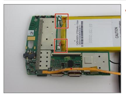
Locate 3 wires(red, blue and black) that connect the motherboard and the battery.
