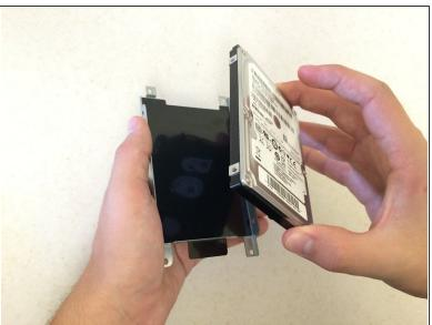
Remove the hard drive from the bracket.
