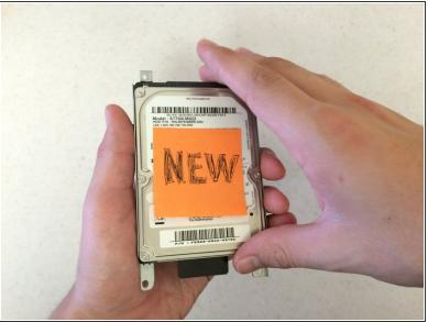
Insert the new hard drive into the bracket.
