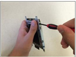
Remove the four screws on the side of the hard drive and bracket.
