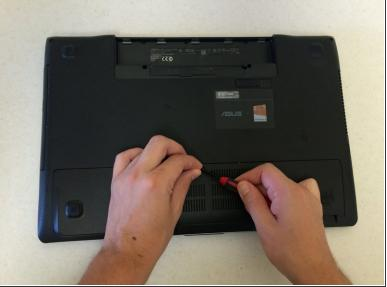
Use the screwdriver to remove the rubber cap on the top of the backplate.
