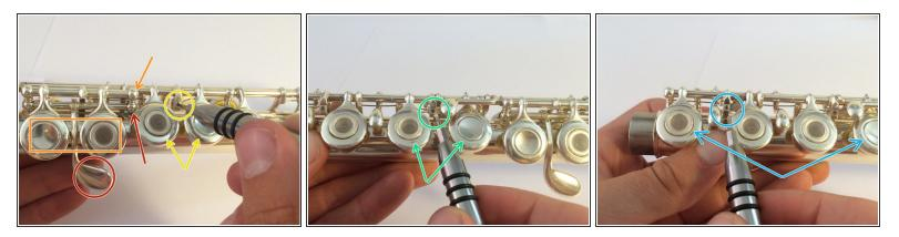
When putting your flute back together, some keys may seem either too easy or to hard to press. This is related to the tightness of the screws in the rails, as well as small screws between finger keys that have not yet been mentioned.
