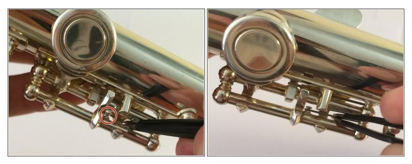
After putting back the inline G keys, make sure to put back the spring behind the peg.
