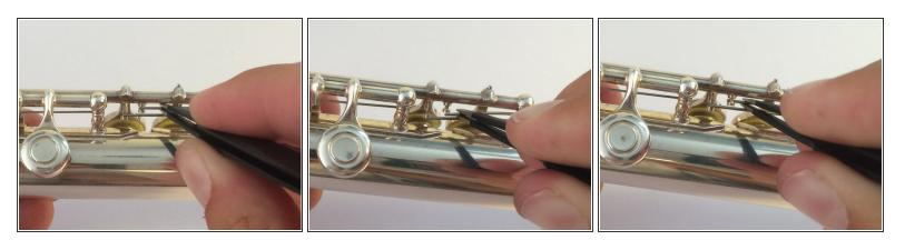
After putting the screws back, fix the springs that connect to the trill keys.
