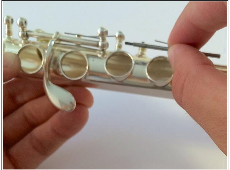
**⚠** Be careful when removing this rod! The spring opposing your direction of motion means business! You can use your free hand to hold it out of the way if necessary.
