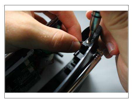
Using the J1 Philip's head screwdriver, unscrew the bolt attaching the antenna to the back panel.
