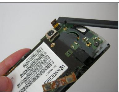
• Place the flat end of the spudger underneath the digitizer connector and pry it up to disconnect it.
