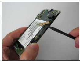
Unclip the two flex cables -- a small one located on the left side on the lower half of the motherboard, and a longer one on the right side, higher up.
