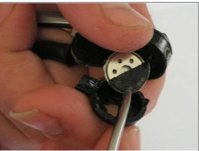
Use Precision Tweezers to remove the protective screen from the front of the speaker unit.
