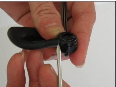
The two snaps that combine with the adhesive to hold the assembly together are located in the neck of the earpiece unit.
