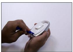
Using plastic opening tool, pry and remove the battery lid.
