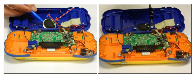
Insert the new speaker into the hatch located in the middle part of the panel using a plastic spudger.
