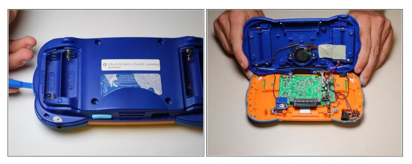
Using a plastic opening tool, separate the two pieces of the case carefully.
