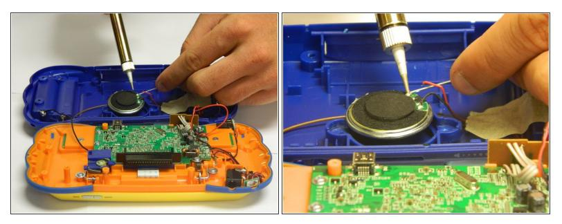
Solder the wires to the appropriate spots on the new speaker, making sure that both wires are properly connected.
