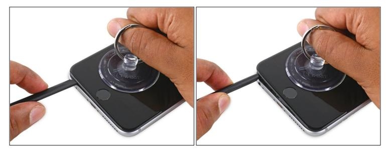
• Twist the spudger to widen the gap between the front panel and the rear case.
