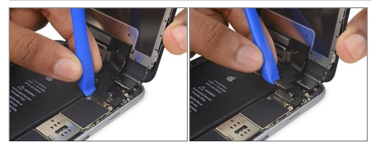
A Be careful to only pry up on the connector itself and not the socket on the logic board.
