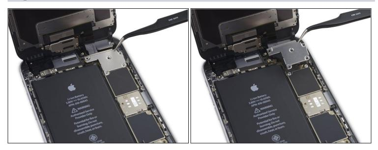
• Remove the display cable bracket.
