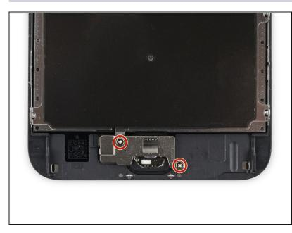
• Remove the two 1.9 mm Phillips screws securing the home button bracket.
