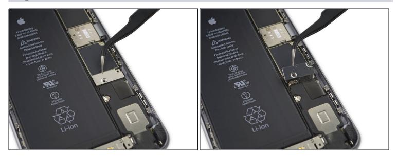
• Remove the battery connector bracket.
