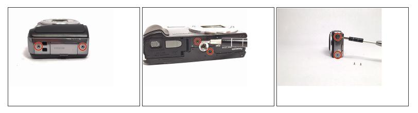
Locate the pair (2) of screws on each side of the camera and remove them. Then locate the pair (2) of screws on the bottom of the camera, located on each side of the tripod screw-in area, and remove them.
