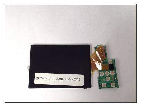
Using your hand, follow the two data-strips that connect the LCD screen to the motherboard and unclip them. Once the data-strips are unclipped, remove them from the motherboard and the screen will be free.
