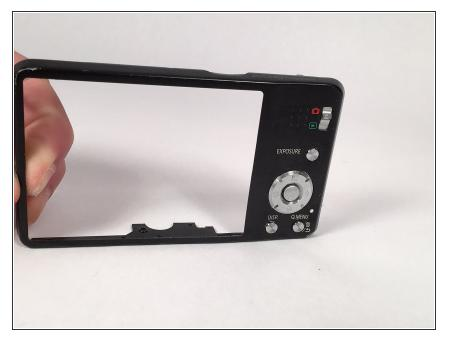
Using the plastic prying tool, remove the cover of the camera that is on the same side as your LCD screen. This cover should come off relatively easily, and will expose the motherboard that the screen is connected to.
