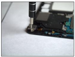
• Remove the two 10mm Phillips #000 screws that hold the left speaker.
