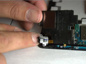
Pull the speaker out and lay it to the side until the rest of the connections are disconnected.
