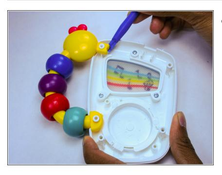
With the help of a plastic opening tool, remove the handle of the device.
