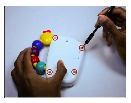
Using a Philips #1 screwdriver, unscrew the four highlighted screws on the back side of the device.
