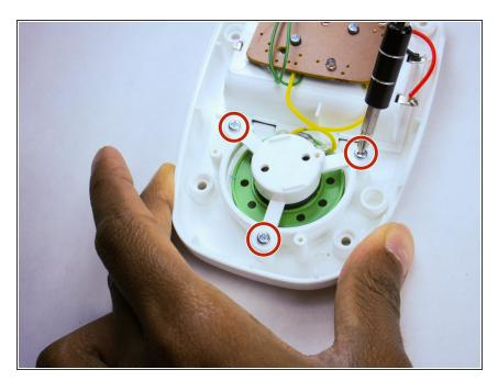
Once the chip is off, loosen the screws on the plastic enclosing the speakers.
