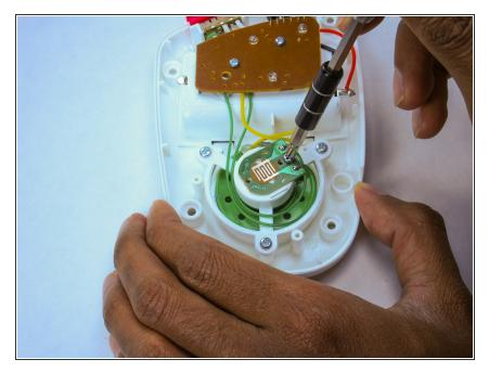
Loosen the screw on the chip with a screwdriver.
