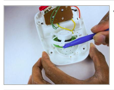
Using the plastic opening tool, pop the plastic enclosing off.
