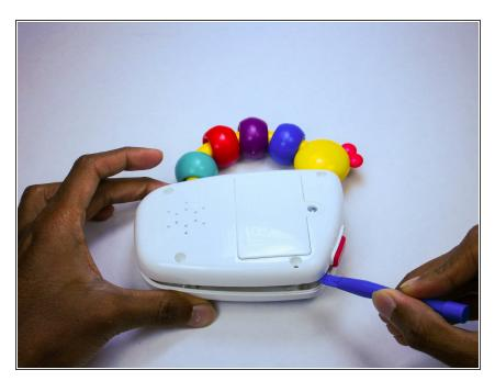
Once unscrewed, pop the back of the device off using the plastic opening tool.
