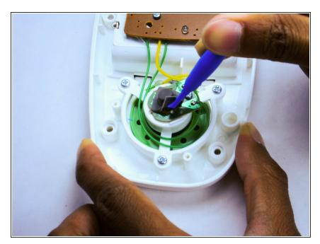
Remove the rubber button by popping it out with the plastic opening tool.
