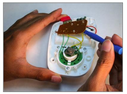
Using a plastic opening tool pop the light panel off. Be careful as to not rip any of the wires from the panel.
