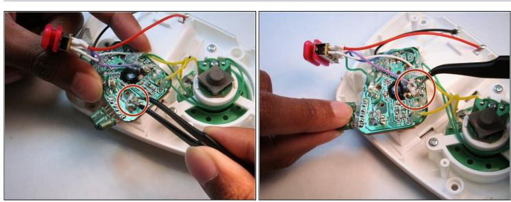
• Carefully pull the LED lights off with a pair of <u>tweezers</u>. Once off, put in and connect a replacement.
