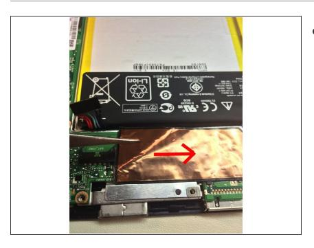
Next step is to peel off the copper tape. Left to Right
