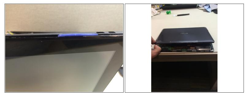
Insert a pick, and slowly go around the edge of the tablet to loosen the back shield
