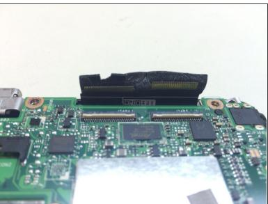
Next step is a little tricky. We have to disconnect the digitizer. ! Be very careful you don't ruin the closing mechanism. Simply pull back and pull slowly until the connection comes out.
